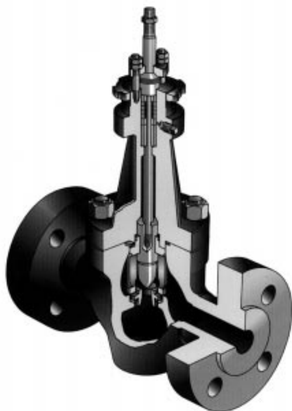
BV502 series valve fitted with contour trim and normalising bonnet
