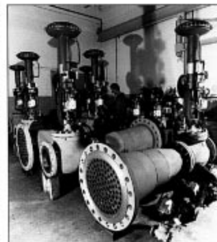
Valves with low noise trim and outlet silencers destined for a desalination plant in the Middle East.
